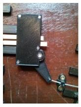
The switch mechanism operates both blades via a single push-pull rod, connected to a modified door bolt. The turnout is fixed to the boards with turn buckles, and the usual Jackman track joiners.
